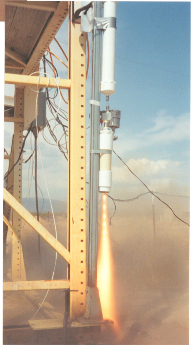
Photo 6. (Above) Mark Ventura's 50 pound thrust, 85% hydrogen peroxide/polyethylene hybrid undergoing test. All the major components were fabricated from PVC pipe.
