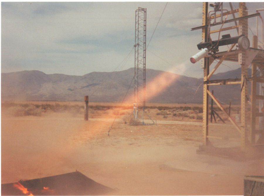
Photo 4. (Left) Scott Claflin's 1600 pound thrust lox/alcohol engine running for 7 seconds. The black square burning in the lower left is the particle board flame deflector used to reduce the dust kicked up. It did not work well.
