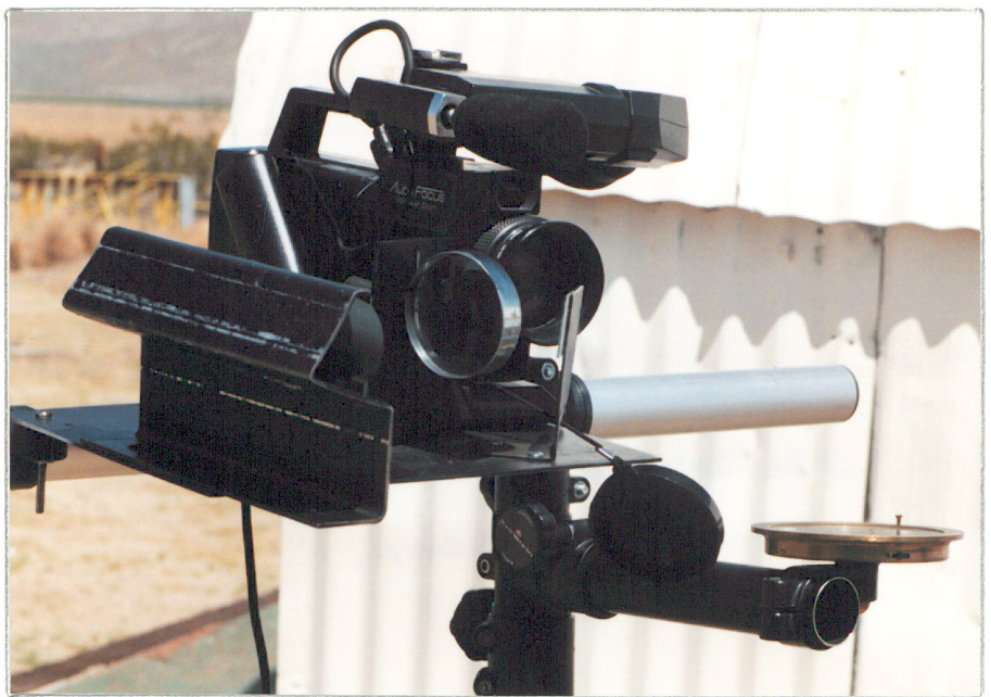
Photo 2 - The video phototheodolite built by Bill Colburn and used at the 23 April, 1994 firing.
