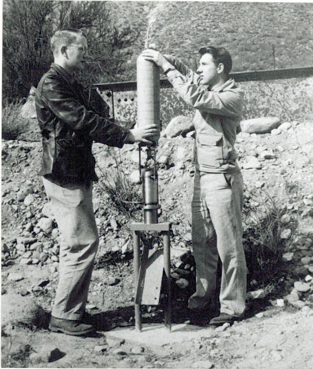
Photo 1 - Lee Rosenthal (left) and David Elliott set up the propulsion unit in the test stand for one of the first static tests. The facility nitrogen pressurization is being attached. The “I” beam in the background provided protection for the test crew.
