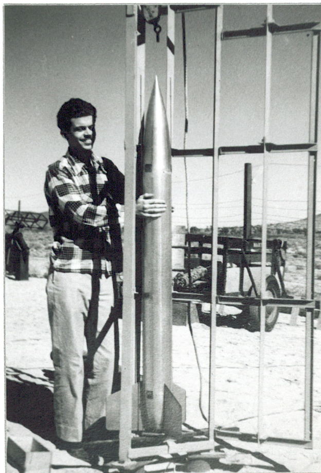
Photo 10 - Glen Maxon conducting a fit check of the rocket in the launch tower during final rail adjustments.
