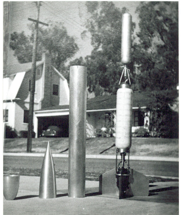
Photo 6 - All the major subassemblies of the hydrogen peroxide monopropellant rocket.
