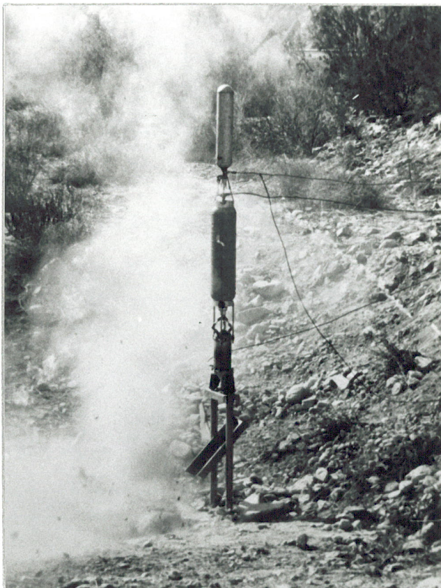
Photo 4 - Static test Number 6 run on 27 March, 1949. This test included the flight pressure bottle and valve assembly.
