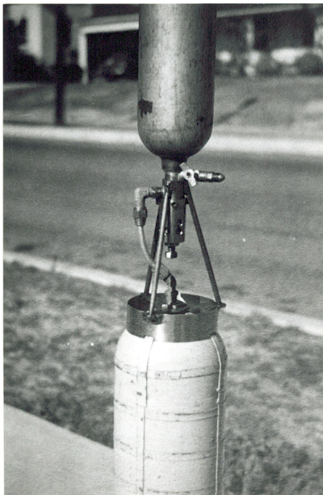
Photo 3 - Close up of the pyrotechnically actuated high pressure nitrogen valve installed between the peroxide tank and the flight nitrogen bottle. The struts held the pressure bottle in place. The bolt head at the lower end of the pyro valve was used to push the solid propellant capsule against the valve stem closing off the high pressure nitrogen and keeping the peroxide tank vent open. The valve opened when the capsule was burned.
