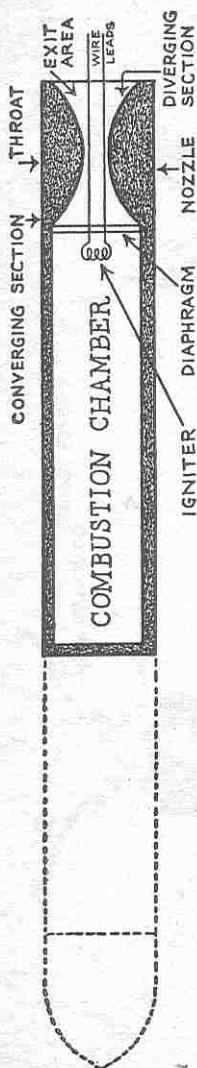
TYPICAL ROCKET MOTOR FOR A SOLID PROPELLANT
