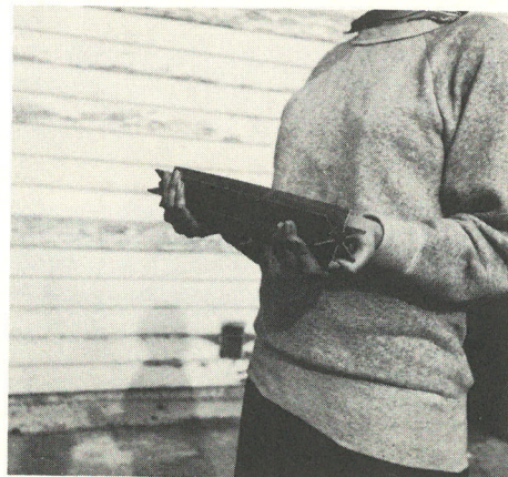
STAR GRAIN MANDREL. Protruding from the hexagonal stock are six one-eighth inch vanes. Mandrel is seventeen inches long.
