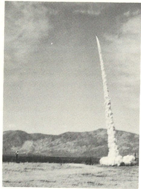
STANDARD BETA ROCKET TAKE-OFF, using zinc and sulfur in a weight ratio of 3:1, packed by hand.
