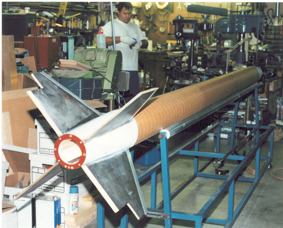
The skin is mounted on the rocket structure in this photo. After all internal components were installed and leak tested, the skin was installed for the last time.
