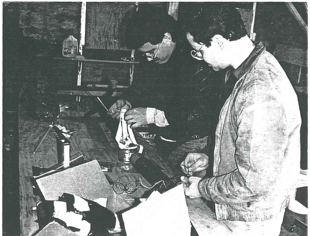
Figure 5 - Jim and Alan work to complete final preparations on the high power rocket to test an Adept Electronics recording altimeter and parachute deployment system.
