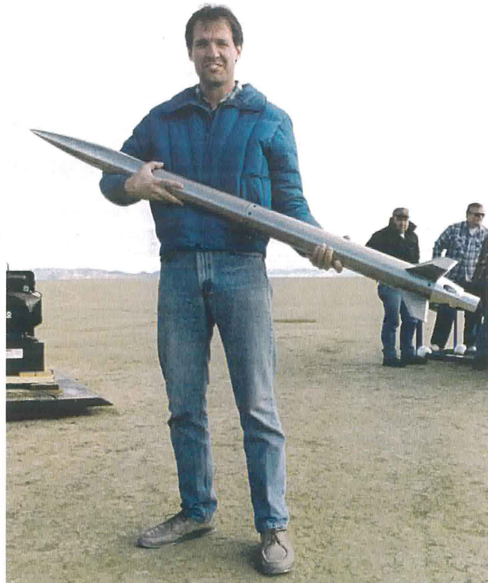
Above - Mike Henkoski hold up the video package he put together on such short notice. The oval hole in the boat tail is the port through which the camera viewed the ground.
