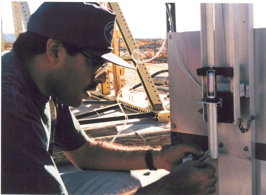
Below - Rene Caldera prepares to test his micro hybrid on an instrumented test stand.
