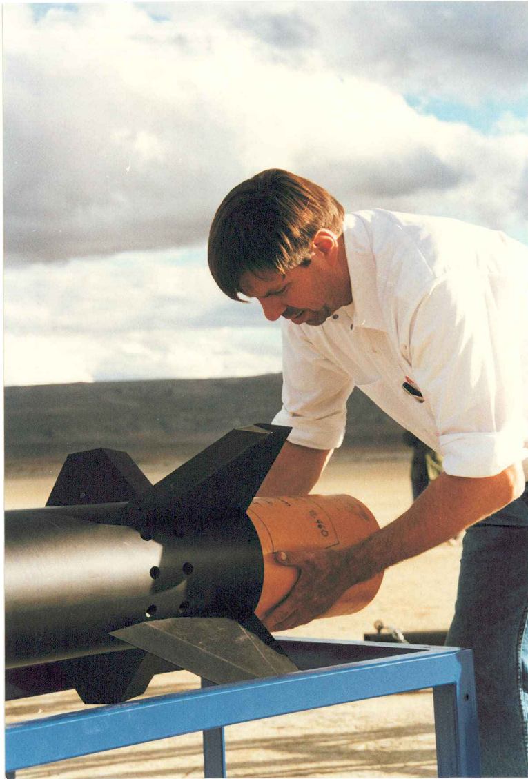
Left - George Garboden installs a lightly greased grain in the lower end of the motor case.
