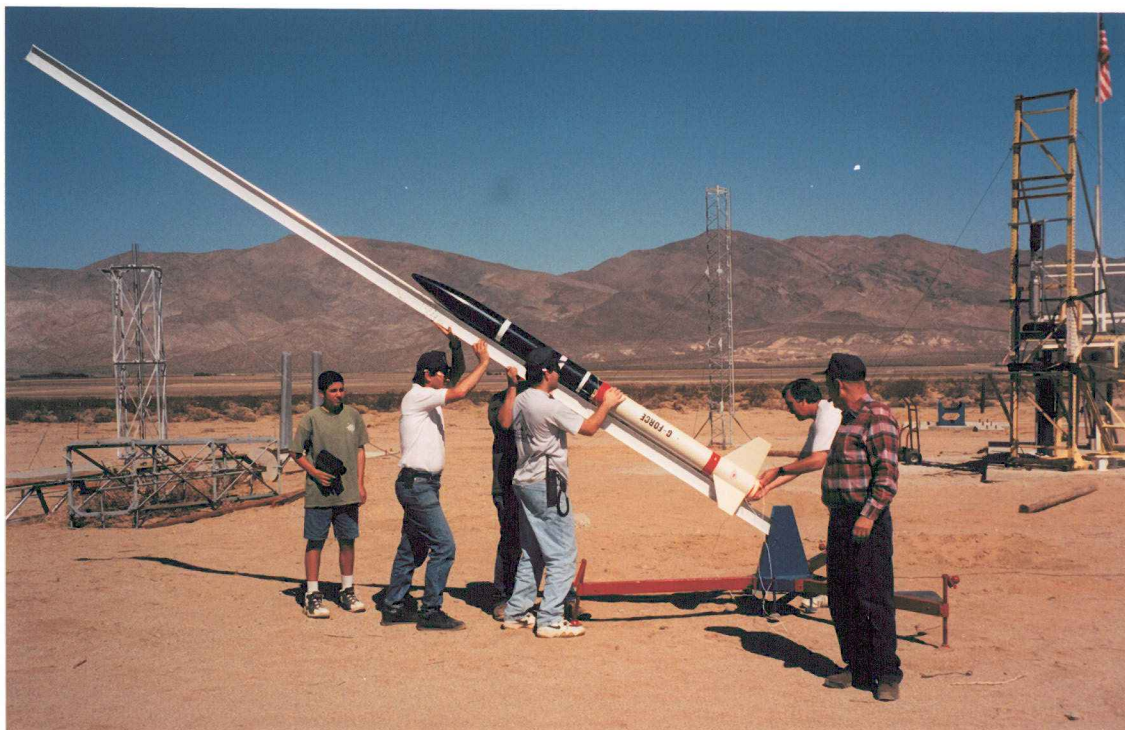
Sledgehammer II is loaded on its launcher and raised to the firing azimuth.
