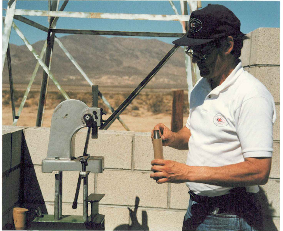
Above - Steve Majdali loads black powder rockets in the solid propellant processing area (SPPA).
