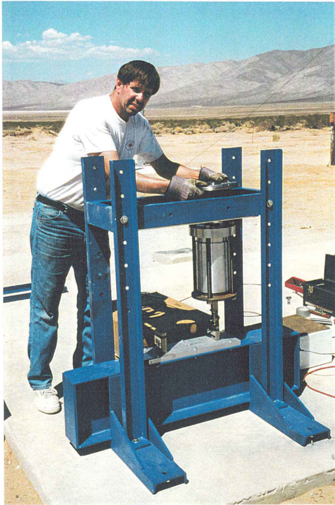
Left - Propellant characterization testing was conducted with subscale 5-inch diameter hardware. Here, George Garboden installs the test article in the static test stand at the MTA.
