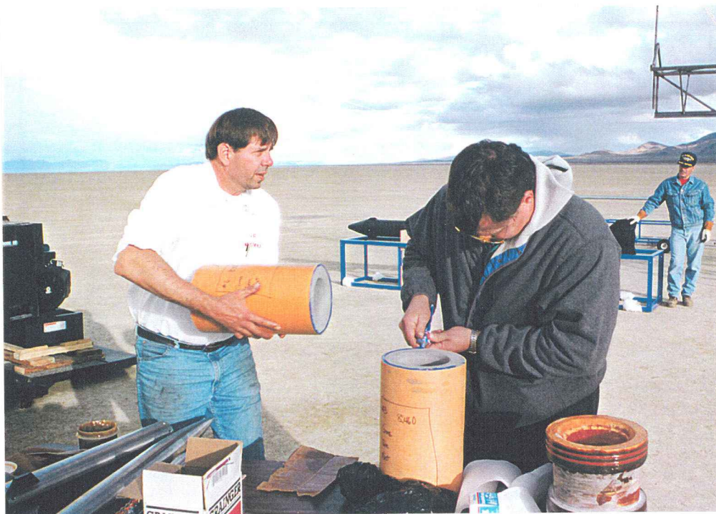
The propellant grains are prepared by George Garboden and Brian Wherley for installation in the motor case.
