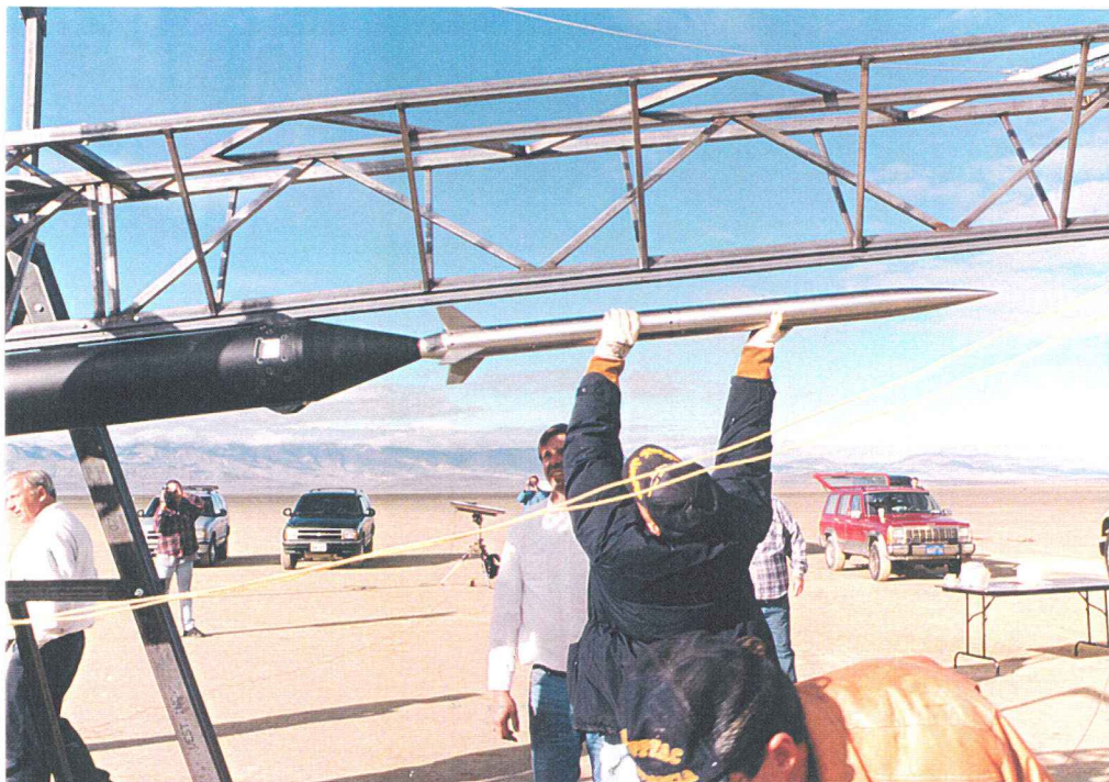
The booster has been loaded on the rail and the dart is set in place.
