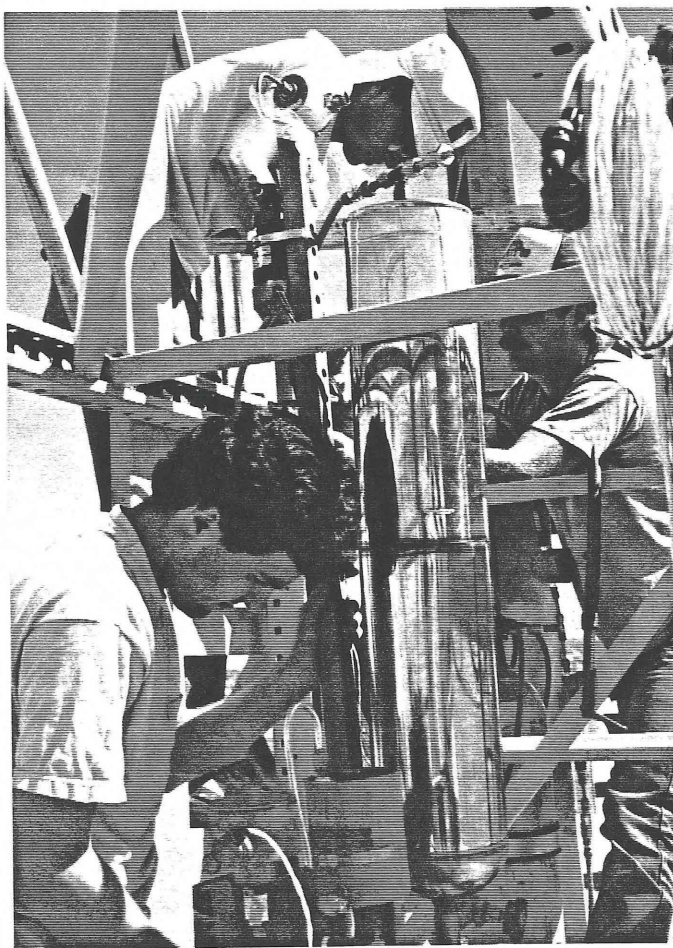
Mark Grant (top) and Gary Perkins (right) assist in installing the LOX tank and connecting the helium pressurant.
