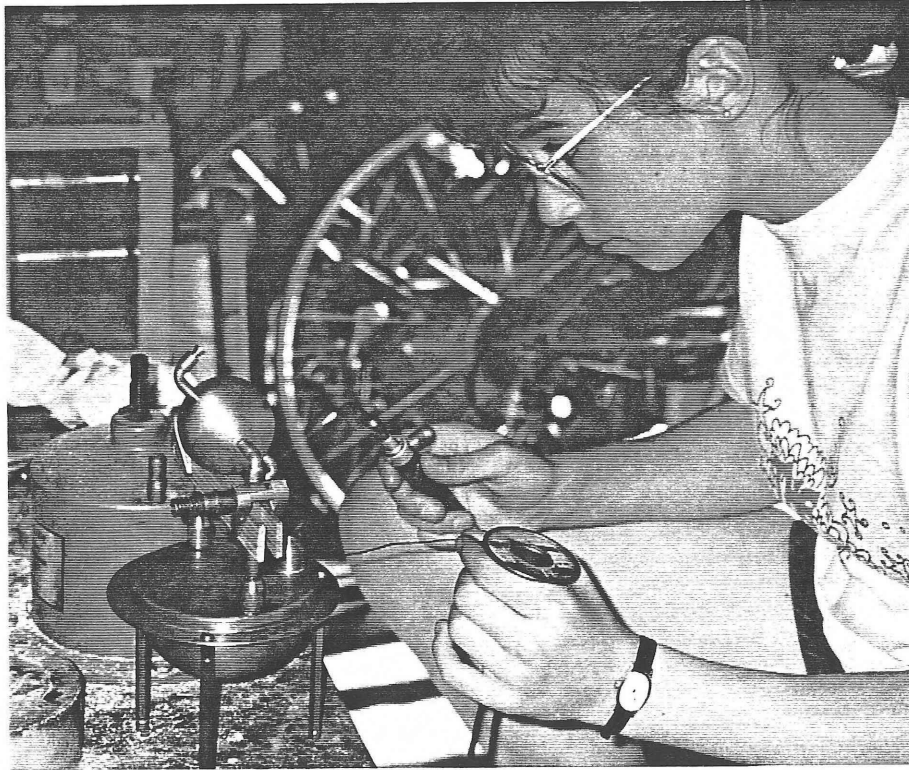
Finishing the assembly by soldering the steam supply and pivot support tubes in place on top of the boiler.
