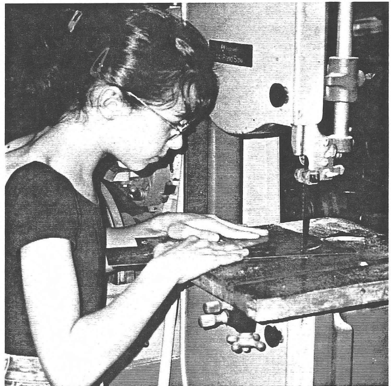
Cutting the copper plate to make the top of the boiler
