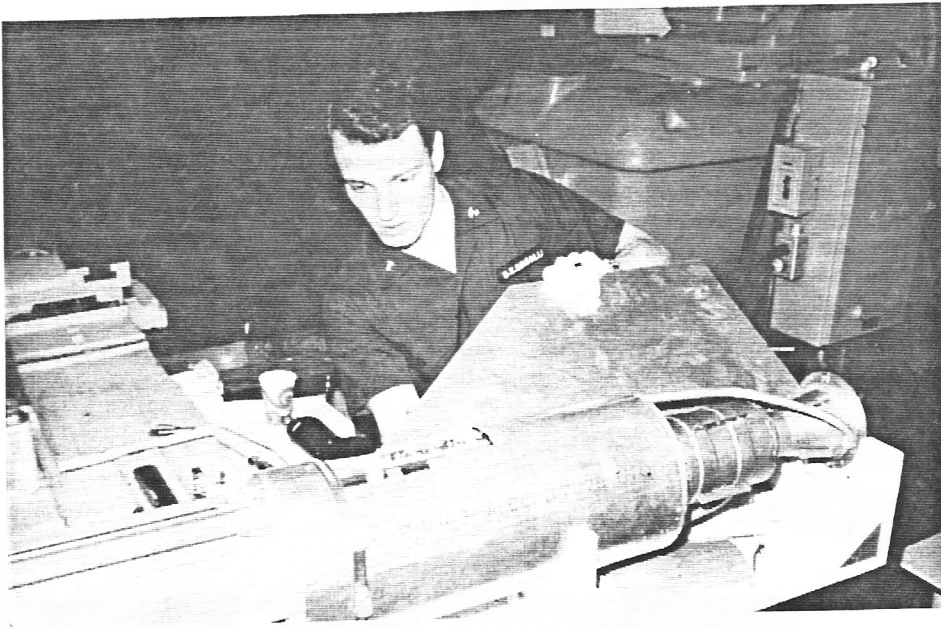
ABOVE - D. Crisalli fitting fins to the tail assembly.
