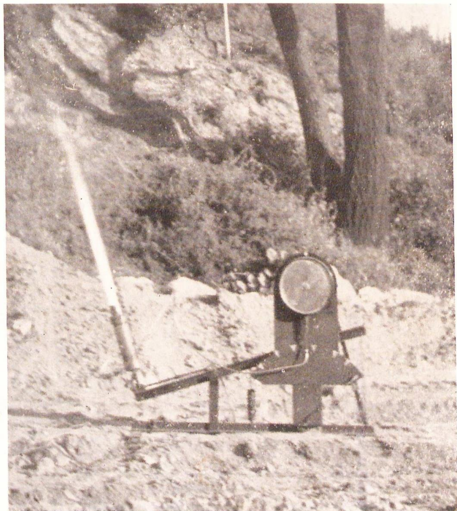
Reaction Research Society Solid Liquid Engine No.1 in operation. Engine was making over 25 pounds thrust when photograph was taken.
