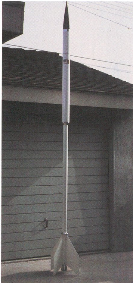
The ER-15 (Experimental Rocket 15). The 2.5 inch diameter motor held 25 pounds of propellant and produced 1500 pounds of thrust.
