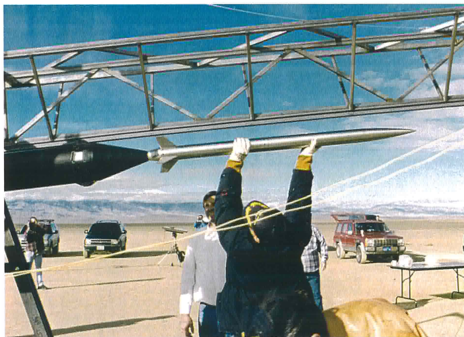
The booster has been loaded on the rail and the dart is set in place.
