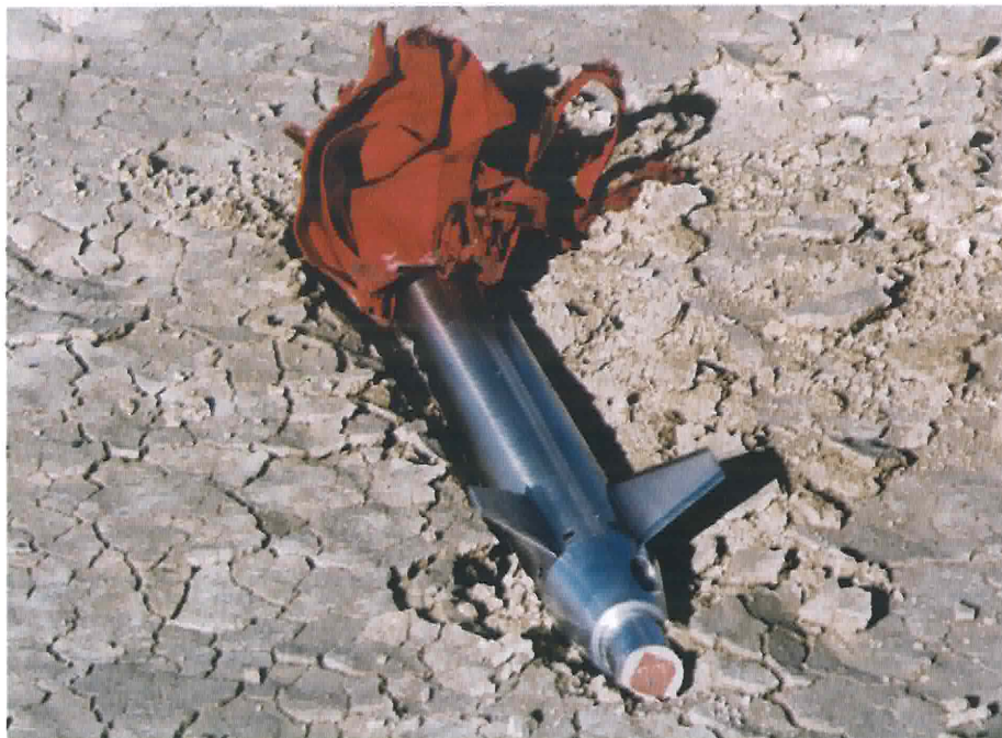
The dart as it was found stuck in the surface of the lake still working after its flight to the edge of space.
