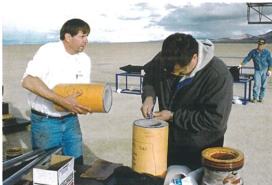
The finished propellant grains are prepared by George Garboden and Brian Wherley for installation in the motor case.
