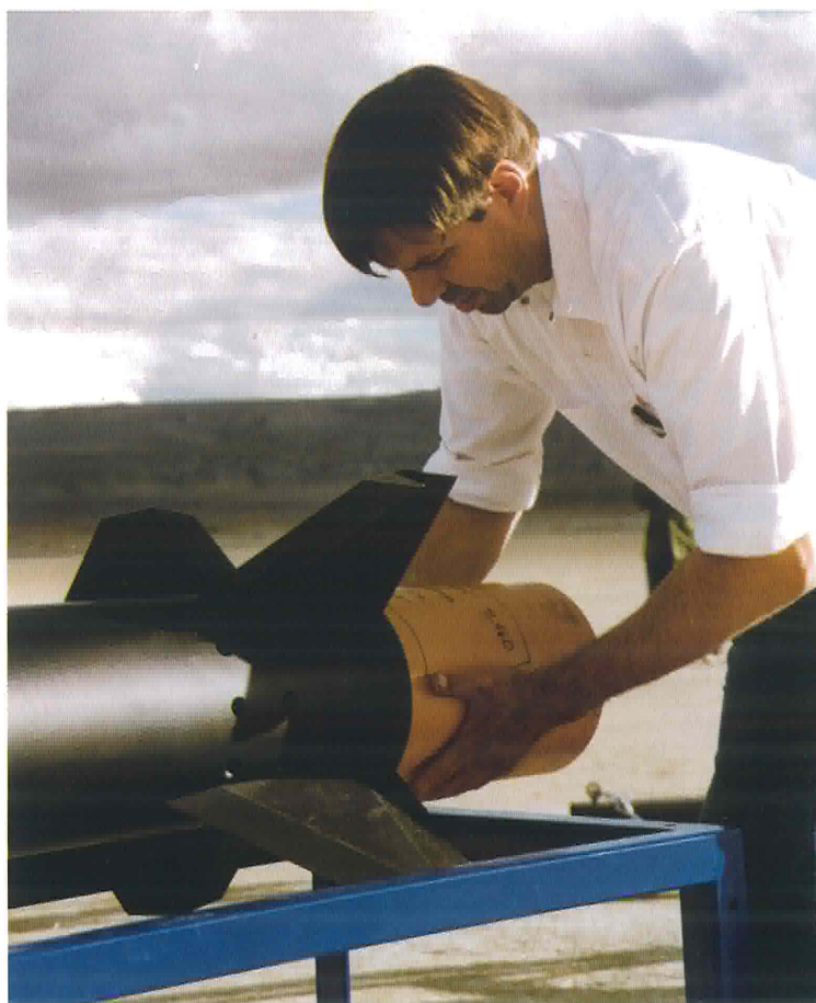
George installs a lightly greased grain in the lower end of the motor case.
