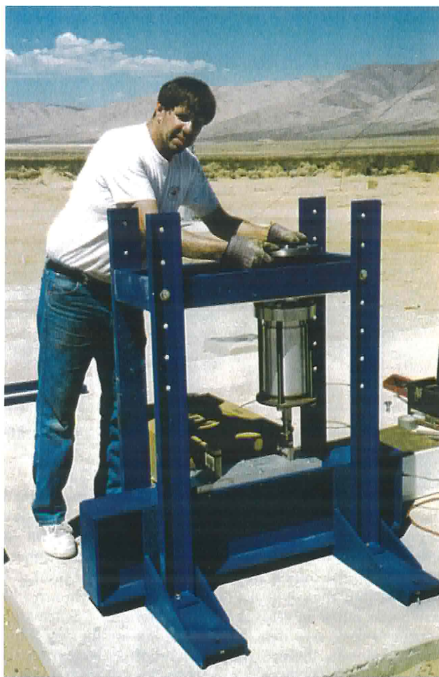
The initial propellant characterization testing was conducted with subscale 5-inch diameter hardware. Here, George Garboden installs the test article in the static test stand at the Mojave Test Area.
