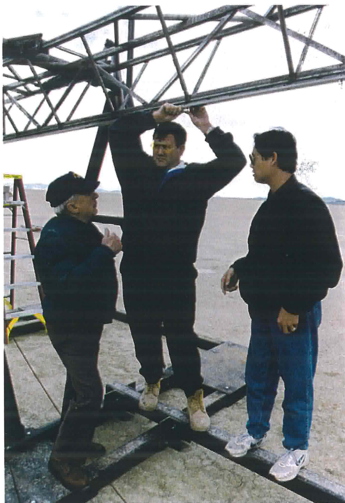
From left: Cris Crisalli, Brian Wherley, and Craig Tang fit and shim the rail to the launcher.
