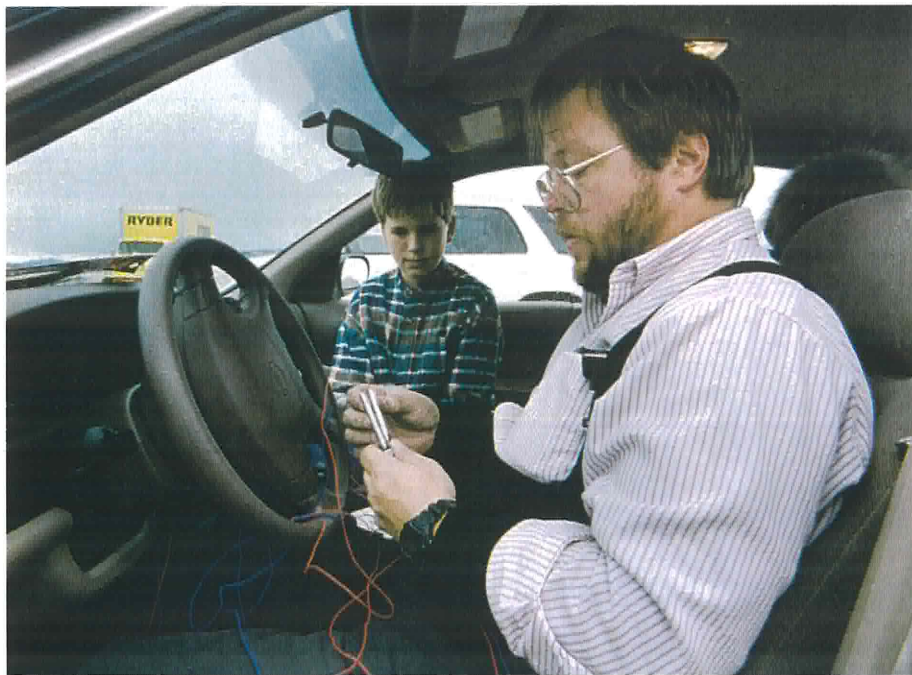
Niels Anderson shows Clayton Mosier how to make igniters. Niels had to do this in the car with the heater running to get the epoxy to cure in the cold weather!
