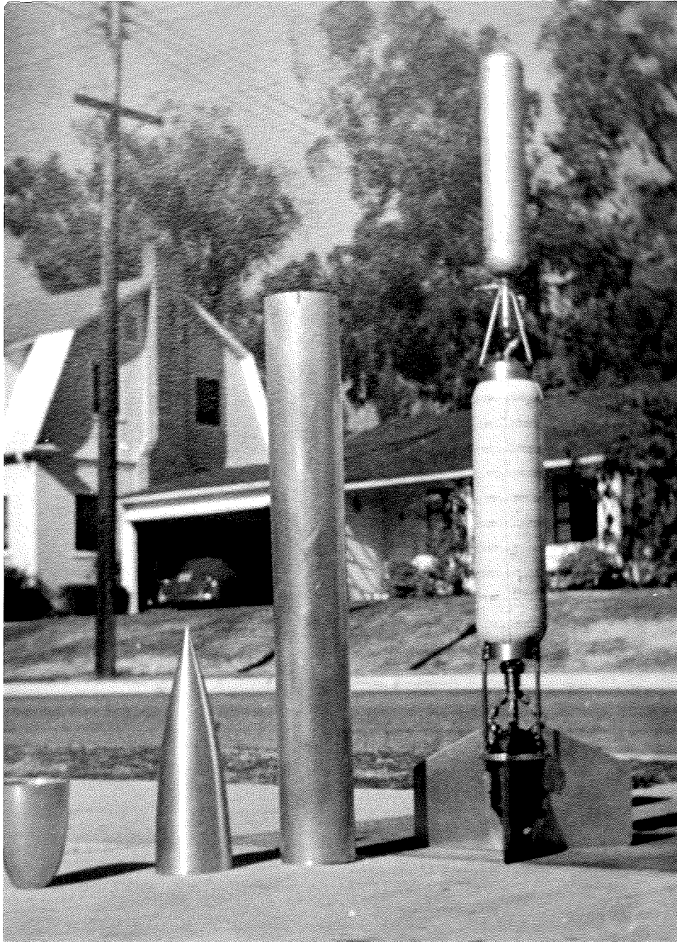
All major components and subassemblies of the hydrogen peroxide monopropellant rocket.
