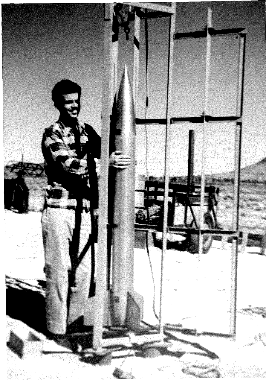
Glen Maxon conducting a fit check of the rocket in the launch tower during final rail adjustments.
