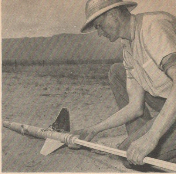
Full safety precautions are observed during the critical period when the solid fuel is tamped into place
